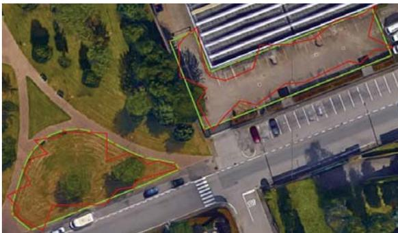
The **RED** route is obtained joining GPS points measured with a Smartphone, the **GREEN** one with STONEX S5 GNSS connected with the smartphone.
