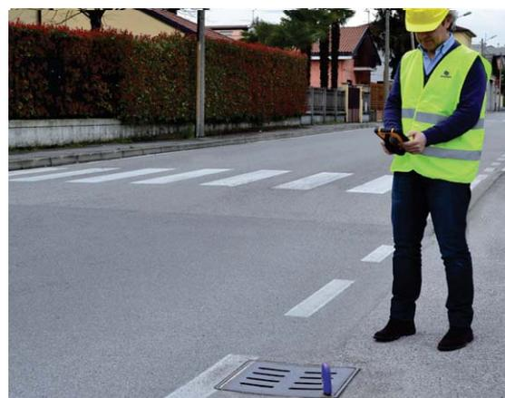
Tested on April 21st, 2016 - S5 + S4C CUBE SW + external GNSS antenna p/n 30-350161 - Corrections received using the integrated GPRS modem of S5
